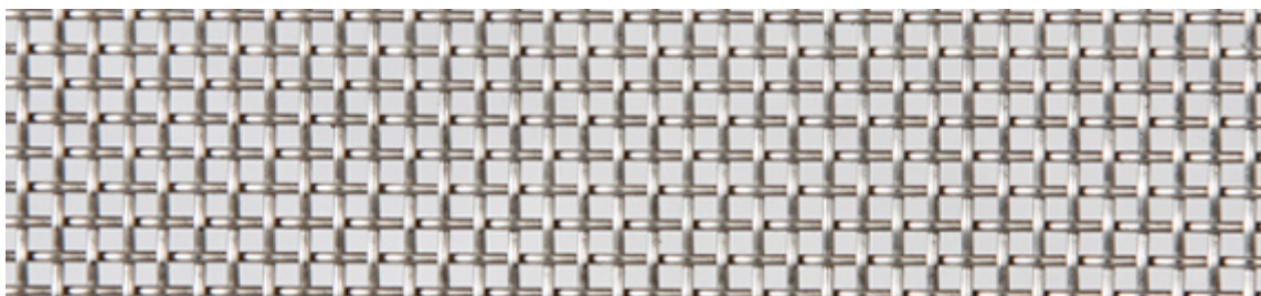
Figure 3 Close up of proposed radiation screen mesh. Wire diameter typically 0.3mm at 2mm centres
